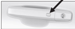
1 st Row Passive Entry button will only unlock the front row doors
