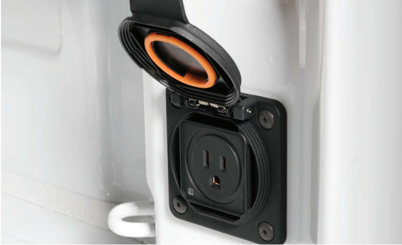
Standard 120-volt power outlet in bed
